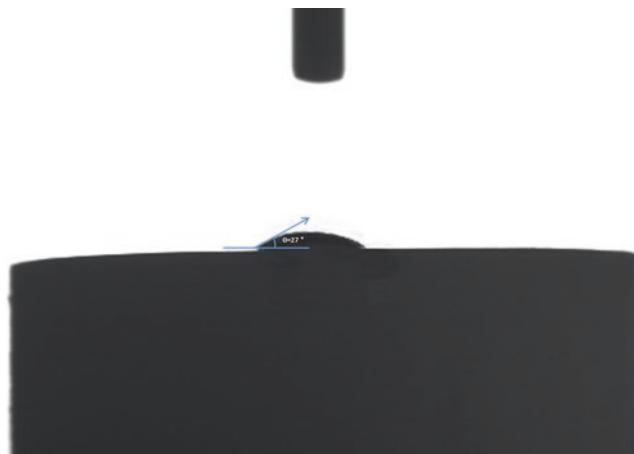
Fig. 1 The water contact angle (WCA) of Au substrate is 27^\circ , which shows the surface of Au has a good hydrophilicity, so the lipid vesicles can form planar bilayers on the surface
